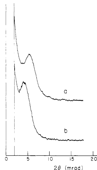
Figure 10. Small-angle X-ray scattering curves measured on the PEO-PI-PEO block polymer complexed with NaSCN: (a) as cast from benzene-methanol solution, (b) recrystallized by slow cooling from 470 K to room temperature.
